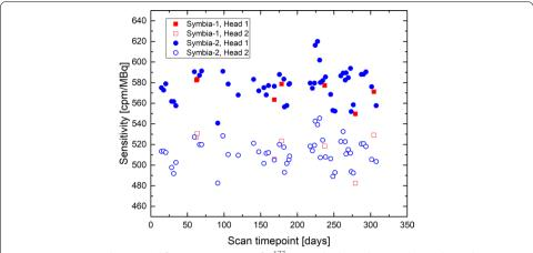
**Fig. 5** Sensitivity as determined from static images of a <sup>177</sup>Lu standard. Head 1 was always above the patient board, while head 2 was below and therefore the sensitivity was reduced due to attenuation in the patient board
