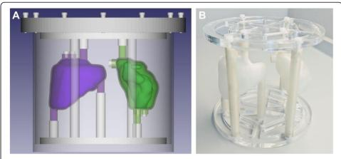
Fig. 1 Two-organ ICRP 110 phantom. A Computer-aided design (purple: one-compartment spleen, green: two-compartment kidney). B 3D printed phantom inserts mounted in the support frame
