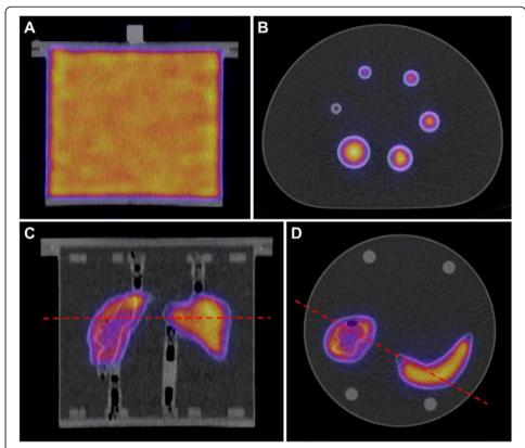
**Fig. 3** Example SPECT/CT reconstructions for a Siemens Intevo Bold system. **A** Coronal view of Jaczszak phantom. **B** Axial view of NEMA phantom. **C** Coronal view of Two-Organ (kidney and spleen) phantom. **D** Axial view of Two-Organ phantom. The red lines indicate the position of the axial cut for the Two-Organ phantom
