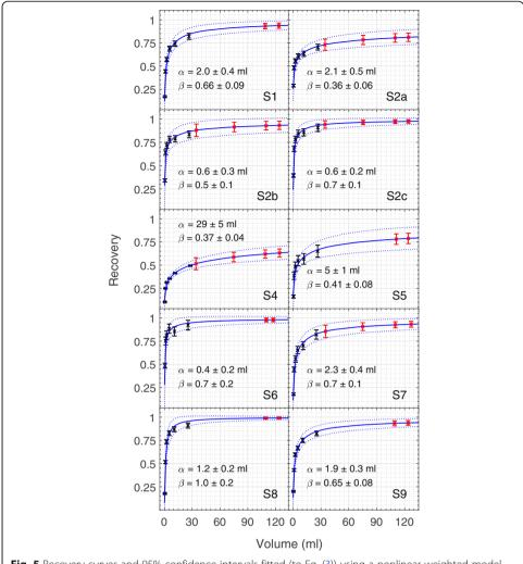
**Fig. 5** Recovery curves and 95% confidence intervals fitted (to Eq. (3)) using a nonlinear weighted model for the calculated NEMA spheres recovery coefficients (black). The fitted recovery coefficients calculated for the validation data are shown in red
