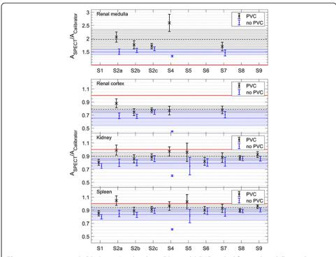
**Fig. 6** Activity ratios with (black cross) and without (blue circle) PVC applied for renal medulla, renal cortex, kidney and spleen inserts (top to bottom). For each case, the horizontal line shows the average ratio across all setups with the shaded area showing the region within one standard deviation, whilst the red line represents 100% accuracy. Note the different vertical scale for the renal medulla
