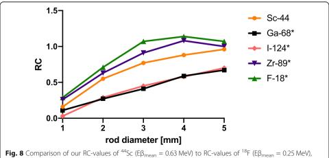
**Fig. 8** Comparison of our RC-values of "Sc ( $E\beta_{mean} = 0.63$  MeV) to RC-values of "F ( $E\beta_{mean} = 0.25$  MeV),  $^{89}$ Zr ( $E\beta_{mean} = 0.40$  MeV),  $^{124}$ l ( $E\beta_{mean} = 0.82$  MeV), and  $^{68}$ Ga ( $E\beta_{mean} = 0.83$  MeV) by Disselhorst et al. 2010 (\*). (reconstruction algorithm: 3D-OSEM/MAP)
