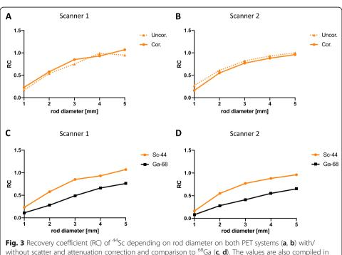
**Fig. 3** Recovery coefficient (RC) of "Sc depending on rod diameter on both PET systems (**a**, **b**) with/ without scatter and attenuation correction and comparison to <sup>68</sup>Ga (**c**, **d**). The values are also compiled in the supplementary material (Table S2). Uncor. without scatter and attenuation correction, Cor. with scatter and attenuation correction
