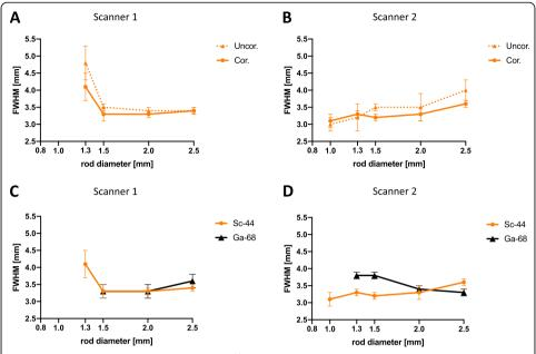
**Fig. 6** Full width at half maximum (FWHM) of <sup>44</sup>Sc depending on rod diameter on both PET systems (**a, b**) with/without scatter and attenuation correction and comparison to <sup>68</sup>Ga (**c, d**). Plotted are the calculated FWHM values with their calculated errors. The values are also compiled in the supplementary material (Table S4). Uncor. without scatter and attenuation correction, Cor. with scatter and attenuation correction
