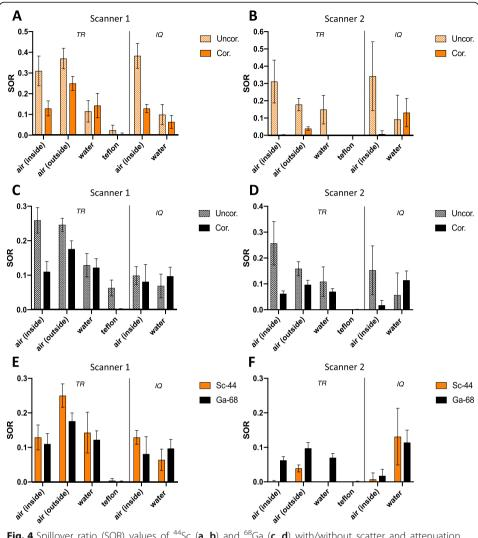
**Fig. 4** Spillover ratio (SOR) values of <sup>44</sup>Sc (**a**, **b**) and <sup>68</sup>Ga (**c**, **d**) with/without scatter and attenuation correction using three-rod (TR) and image quality (IQ) phantom on both PET systems and its comparison (**e**, **f**). Plotted are the calculated SOR values with their calculated errors. The values are also compiled in the supplementary material (Table S3). Uncor. without scatter and attenuation correction, Cor. with scatter and attenuation correction
