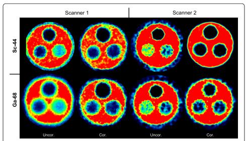
**Fig. 5** Transaxial slides of the three-rod phantom with <sup>44</sup>Sc (first row) in comparison with <sup>68</sup>Ga (second row) on both PET systems. A air, B water, C Teflon, Uncor. without scatter and attenuation correction, Cor. with scatter and attenuation correction
