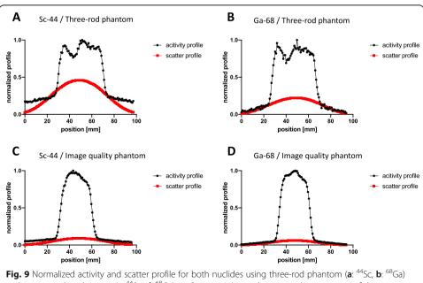
**Fig. 9** Normalized activity and scatter profile for both nuclides using three-rod phantom (**a**: <sup>44</sup>Sc, **b**: <sup>68</sup>Ga) and image quality phantom (**c**: <sup>44</sup>Sc, **d**: <sup>68</sup>Ga) on Scanner 2 (normalization to the maximum of the shown projection)
