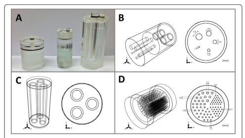
**Fig. 2** The phantoms being used **(a)**. Schematic structure of image quality phantom **(b)**, three-rod phantom **(c)**, and Derenzo phantom **(d)**
