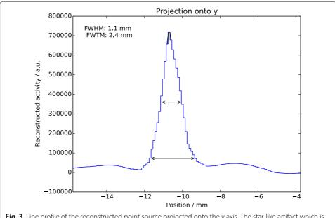
**Fig. 3** Line profile of the reconstructed point source projected onto the *y* axis. The star-like artifact which is aligned with the *x* axis creates an excess in activity at the peak of the profile boosting the spatial resolution
