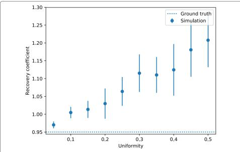
**Fig. 6** Simulated recovery coefficient of the 5-mm rod as a function of the uniformity. The ground truth for the recovery was 0.95. The simulated recovery coefficients are always larger than the ground truth and increase with increasing variance (i.e., larger uniformity values)
