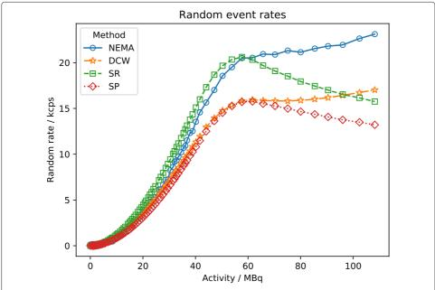
**Fig. 5** Comparison of different methods for the determination of random event rates. NEMA means a method based on the NEMA standard using Eq. 1, DCW uses a delayed coincidence window, SR is based on the singles rate using Eq. 4, and SP incorporates additional corrections using Eq. 5
