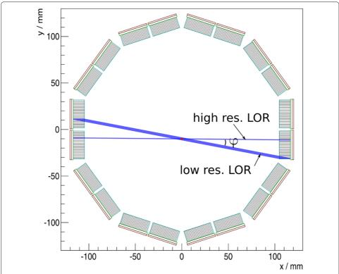
**Fig. 1** Ring geometry that was used for the simulations and the measurement. The blue bands show the parallax error of LORs, which increases approximately proportional to the angle  $\varphi$  to the normal of the block detector
