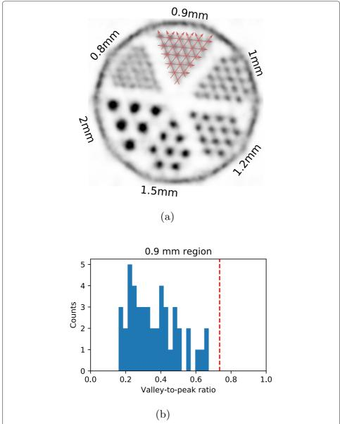
**Fig. 4** Evaluation of spatial resolution using a Derenzo phantom. **a** Reconstruction of Derenzo phantom scan. The labels indicate the diameters and the distance between the rods. The red lines show an example of profile lines which would be used for determination of valley-to-peak ratios to evaluate the spatial resolution. **b** Distribution of valley-to-peak ratios for the region with a rod distance of 0.9 mm. All ratios are below 0.735, which is marked with a red vertical line
