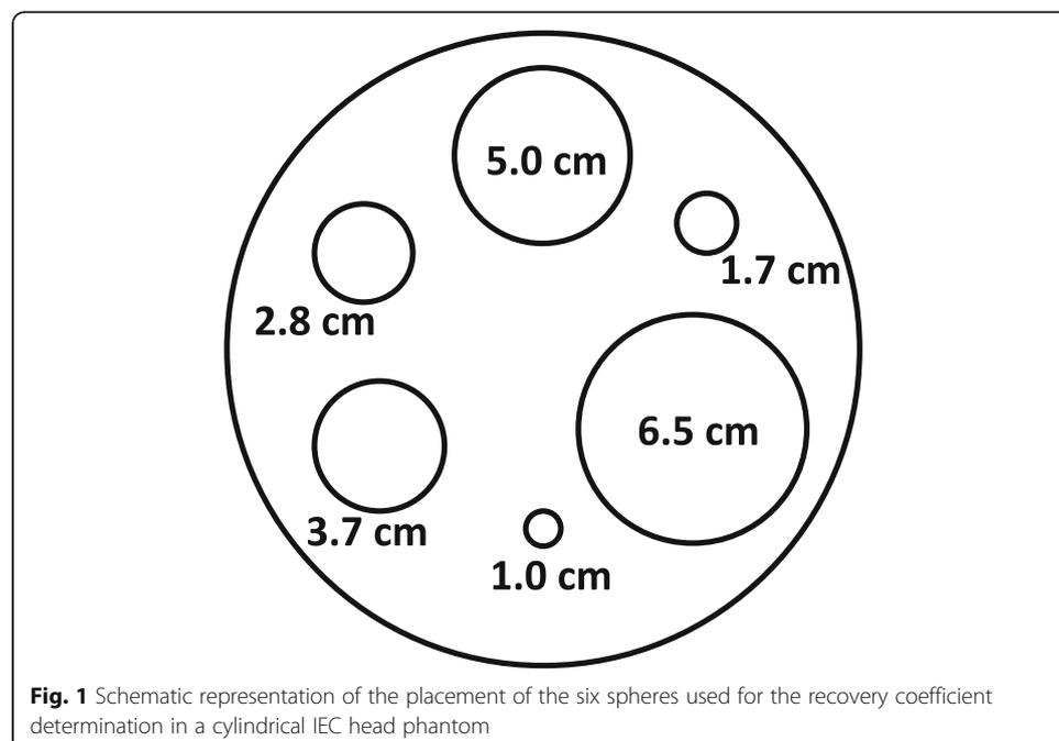
**Fig. 1** Schematic representation of the placement of the six spheres used for the recovery coefficient determination in a cylindrical IEC head phantom
