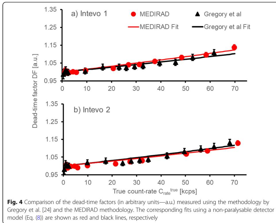
**Fig. 4** Comparison of the dead-time factors (in arbitrary units—a.u.) measured using the methodology by Gregory et al. [24] and the MEDIRAD methodology. The corresponding fits using a non-paralysable detector model (Eq. (8)) are shown as red and black lines, respectively
