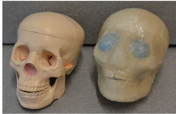
Fig. 1 Commercial skull model (left) which served as a template for creating the bones, and final phantom (right)
