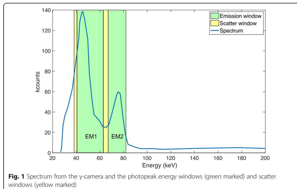
**Fig. 1** Spectrum from the  $\gamma$ -camera and the photopeak energy windows (green marked) and scatter windows (yellow marked)
