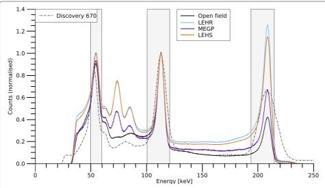
Fig. 8 Spectra of <sup>177</sup>Lu acquired using the open field cover and the three collimators. The spectra are normalised to unity at the 113-keV peak. Differences in peak amplitude may be indicative of septal penetration. A spectrum for the Discovery 670 system is shown for comparison
