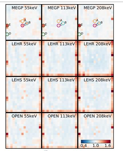
**Fig. 2** Uniformity-correction matrices for <sup>177</sup>Lu for each energy window and collimator (including open field). Values higher than 1.0 correspond to anode elements whose sensitivity is below the detector average. All uniformity matrices are shown using the same colour scale (lower right corner). Circles and letters A–E indicate positions of the five pixels selected for spectral analysis in Fig. 3
