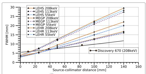
**Fig. 4** System spatial resolution for <sup>177</sup>Lu as a function of the source-collimator distance for each collimator and energy window. The spatial resolution for a conventional gamma camera equipped with an MEGP collimator is also shown, with measured (coloured circles) and simulated (black line) data
