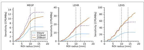
**Fig. 10** Sensitivities for the three collimators as functions of ROI radius, with TEW correction applied for each energy window. The radii corresponding to the source size, and the source size plus 0.5 times the FWHM are shown as vertical dashed lines
