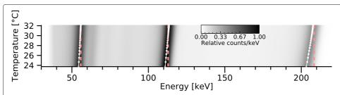
**Fig. 5** Measured <sup>177</sup>Lu spectra as a function of the detector temperature. The grayscale intensity represents the spectral amplitude; each row in the image represents one acquired spectrum. White lines shows the photopeak centres, and vertical red lines indicate the reference photon energies
