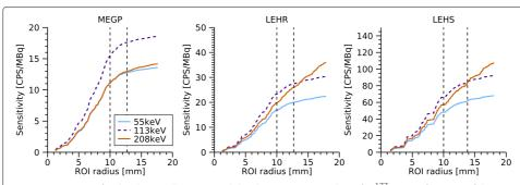
**Fig. 6** Sensitivities for the three collimators and the three energy windows for <sup>177</sup>Lu, as a function of the ROI radius. The radii corresponding to the source size, and the source size plus 0.5 times the FWHM are shown as vertical dashed lines
