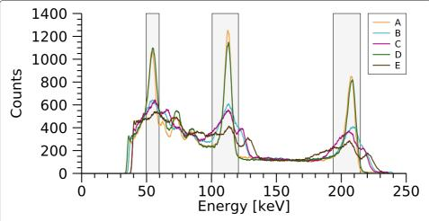
**Fig. 3** Spectra for the five selected pixels for the MEGP collimator, where letters correspond to positions indicated in Fig. 2. Energy windows are shown as grey rectangles. A 1-keV-wide mean-value filter has been applied for noise reduction
