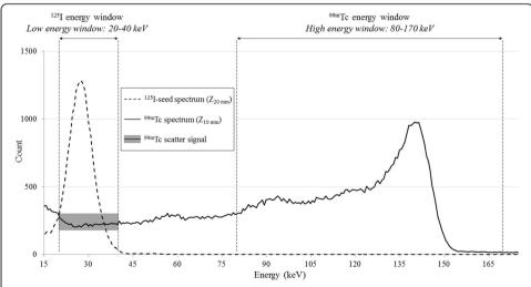
**Fig. 1** Illustration of the EURORAD low (20–40 keV) and high (80–170 keV) energy windows onto the energy spectra of a  $^{99m}$ Tc source and a  $^{125}$ I-seed in a scatter medium performed with the SOE-3214 probe. The sources depths (Z) were considered from the in vitro clinical simulations. These spectra were acquired over 30 s and are presented for 1 MBq activity. The  $^{99m}$ Tc scatter signal corresponds to the  $^{99m}$ Tc signal recorded in the low energy window
