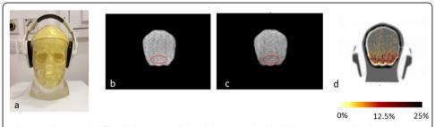
**Fig. 10 a** Photograph of head phantom with headphones in place **b** PET image acquired without the headphones on, **c** PET image acquired with headphones positioned as in **a**, **d** the difference between the image with and without the headphones, as a percentage of the image without the headphones, superimposed onto a CT scan of the phantom with the headphones covering the ears
