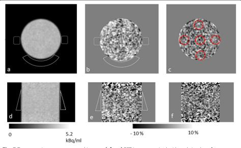
**Fig. 7** Transverse images **a–c**, coronal images **d–f**. **a**, **d** PET image acquired with pads in place. **b**, **e** Difference between PET images with/without pads attached to phantom. **c**, **f** Subtraction of two PET images acquired back to back. Dotted white lines represent the position of the pads in **a**, **b**, **d** and **e**. Dotted red lines in **c** show the positions of ROIs used to make measurements given in Table 1
