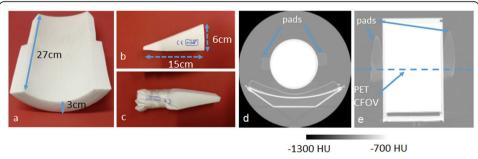
**Fig. 3 a** Pad located under the patient's head in the head coil. **b** A triangular pad (used in pairs) that is positioned between the coil and the head. **c** The same triangular pad compressed with tape to mimic compression when in use. **d** Transverse and **e** coronal CT images in HU showing the location of the pads for phantom assessment (CFOV = centre of the field of view). The blue arrows in **d** and **e** highlight the location of the pads in the CT images
