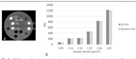
**Fig. 4 a** GE CT image of the electron density phantom labelled with the density of each sample. The image is displayed in HU. **b** HU measured on a GE and Siemens CT image of the phantom
