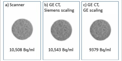
**Fig. 6** Images of the  $^{68}$ Ge daily QC phantom attenuation corrected using **a** CT provided on the scanner, **b** GE CT with Siemens HU to LAC scaling and **c** GE CT with GE HU to LAC scaling. The activity concentration measured in a large ROI located at the centre of the images is shown below each image
