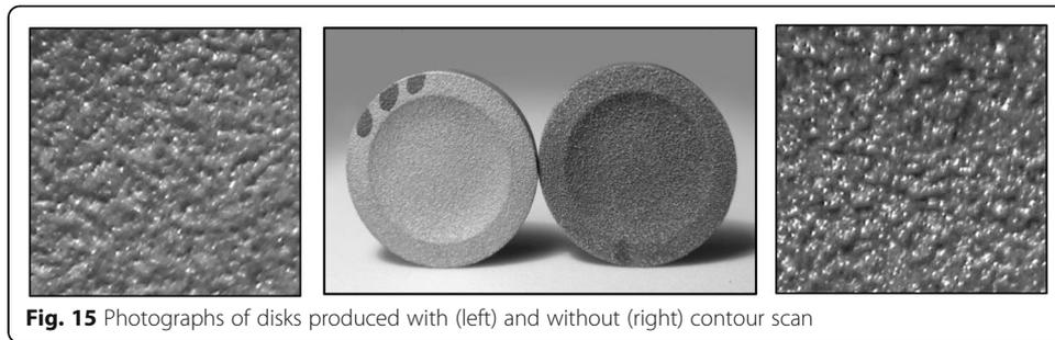
**Fig. 15** Photographs of disks produced with (left) and without (right) contour scan
