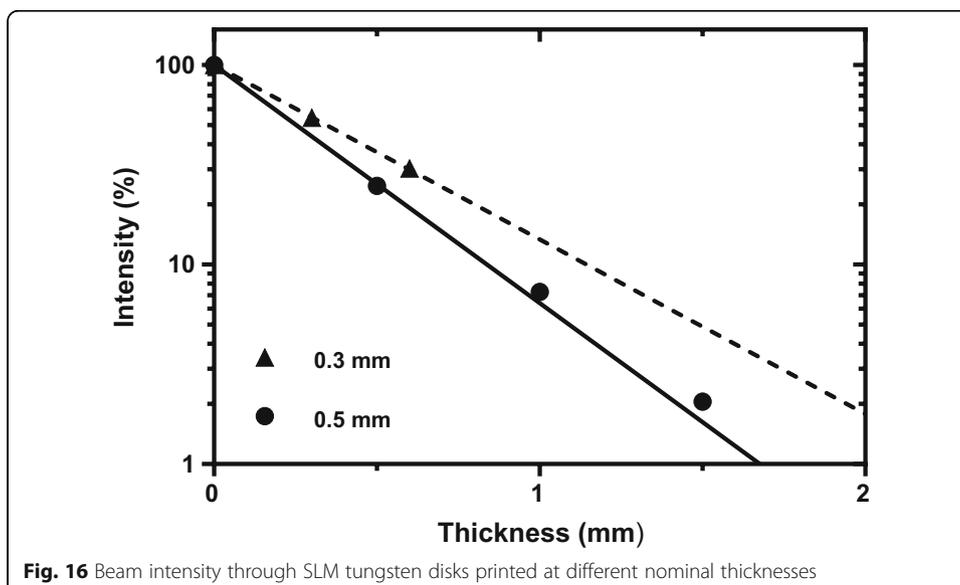
**Fig. 16** Beam intensity through SLM tungsten disks printed at different nominal thicknesses
