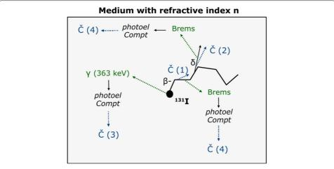
**Fig. 3** Pictorial description of the different processes that can lead to Cerenkov emission. Abbreviations: Brems = Bremsstrahlung, photoel = photoelectron,  $\delta = \delta$  ray,  $\check{C}$  = Cerenkov radiation. Adapted from [69]
