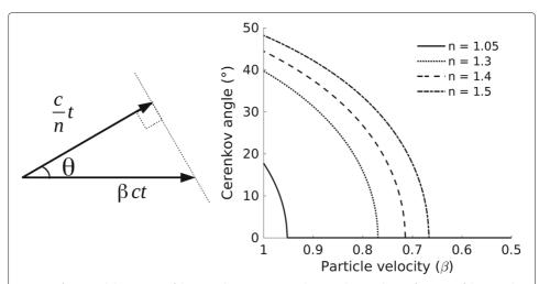
**Fig. 1** Left: Pictorial description of the Cerenkov emission. Right: Cerenkov angle as a function of the particle velocity, for different values of refractive index
