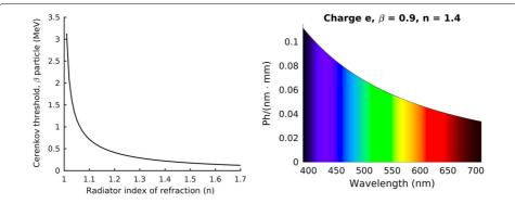
**Fig. 2** Left: Cerenkov threshold as a function of the refractive index of the radiator for a  $\beta$  particle  $(m_0c^2=0.511$  MeV). Right: Number of Cerenkov photons emitted per unit path length and per unit wavelength by a particle with charge e and  $\beta=0.9$  in a medium with  $n(\lambda)=1.4$
