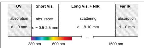
**Fig. 6** Summary of the behavior in tissue of optical radiation of different wavelength, from data in [42]. The penetration depth is indicated as d
