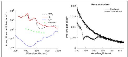
**Fig. 7** *Left*: Absorption spectra of tissue components. Data for both oxygenated and deoxygenated hemoglobin were taken from [44], water data by [45] and melanin data by [46]. *Right*: Monte Carlo simulation of the modification of the Cerenkov spectrum in 1 cm of a typical tissue-like pure absorber (*dotted line*), with the original Cerenkov emission spectrum as a reference
