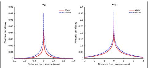
**Fig. 4** Cerenkov emission range, defining the CLI intrinsic limit to the spatial correlation between the source position and the position of production of the Cerenkov radiation, much like the positron range for positron emission tomography. Simulated results were obtained including all the contributions to Cerenkov light production (1–4) of Fig. 3
