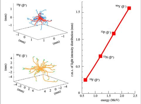
**Fig. 5** *Left*: Cerenkov production range simulated by [32], considering only the contribution of the primary  $\beta$  particles (1) in Fig. 3. *Right*: simulated spread in the Cerenkov light production as a function of the  $\beta$ -particle endpoint energy, for a few radionuclides (both with permission by [32])
