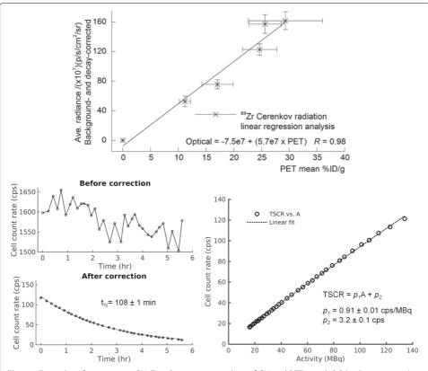
**Fig. 11** Examples of quantitative CLI. *Top*: Quantitative analysis of CLI and PET signals [2] (with permission). *Bottom left*: Decay in time of the count rate due to <sup>18</sup>F measured by the PDPC, before and after data correction [27]. *Bottom right*: Linearity of the Cerenkov count rate in the PDPC with the <sup>18</sup>F activity level, adapted from [69]
