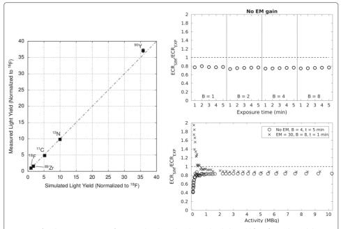
**Fig. 12** *Left*: Relative comparison of measured and simulated Cerenkov light yield for a few radionuclides in water [58] (with permission). *Right*: Simulated over measured Cerenkov count rate with different acquisition settings (top) and as a function of activity, for two combinations of acquisition settings (bottom); both figures were adapted from [125]
