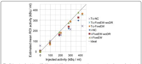
**Fig. 7** Linearity of activities of Tc-99m and I-123 six-compartment phantom: scattering diagram of estimated mean ROI activities for six compartments in image with no correction (NC) and corrected by FiveEW and FiveEW-woDR methods. Tc and I indicate main energy window for radionuclide of interest
