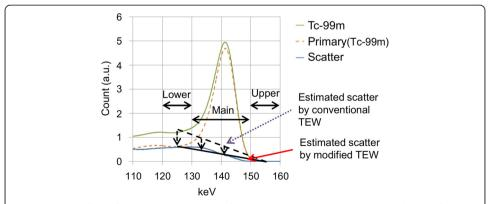
**Fig. 2** Concept of modified TEW method: spectra for Tc-99m and primary (Tc-99m) were obtained from phantom measurement and scatter-free radiation source measurement. Spectrum for "scatter" was calculated by subtracting "primary (Tc-99m)" from "Tc-99m." Conventional TEW method and modified TEW method are described in Eqs. 1 and 6, respectively. Amount of estimated scatter was reduced to acceptable level by taking into account fraction of primary count in lower sub-window
