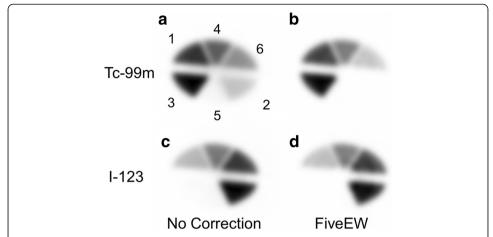
**Fig. 6** Six-compartment phantom images: simultaneous dual-radionuclide images of mixture of Tc-99m and l-123. Tc-99m images with no correction (**a**) and corrected by FiveEW (**b**); l-123 images with no correction (**c**) and corrected by FiveEW (**d**). After scatter correction by FiveEW method, contamination from l-123 in compartment 2 clearly disappeared
