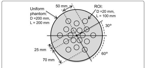
**Fig. 4** Uniform phantom and ROI settings: distances from centre of phantom to ROI centres were 25, 50, and 70 mm. Each ROI had same radius of rotation; they were placed every 60°
