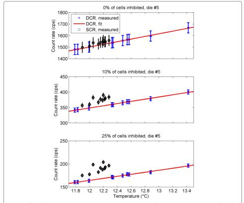
**Fig. 12** Effect of the HDC cells removal algorithm. *Error bars* are taken from Table 2. The *y*-scale is different for each plot, and the dispersion on the *y*-axis of the data related to the source is due to the different attenuation of the light during the acquisition (different thickness of chicken breast, see Fig. 3)
