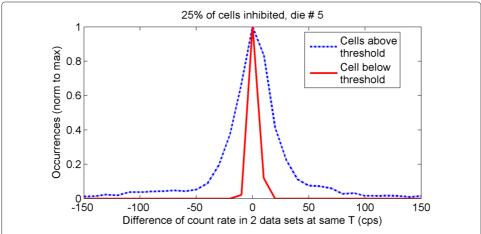
**Fig. 9** Comparison of measurements at same temperature. Distribution of the differences in the count rates measured in two independent acquisitions performed at the same temperature (12.5  $\pm$  0.4 °C), for one central die of the tile
