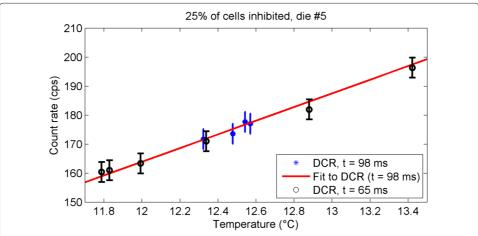
**Fig. 10** Comparison of the dark count rate with different activation time. Dark count rate measured with t = 98 ms (*stars*), expected dark count rate as a function of temperature (*solid line*), data set with t = 65 ms (*circles*)
