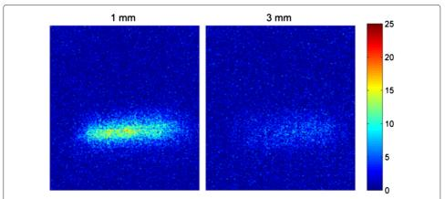
**Fig. 16** Sample images. Images of the capillary tube filled with  $^{90}$ Y placed under slices of chicken breast of 1 mm ( $\mathit{left}$ ) and 3 mm ( $\mathit{right}$ ) thickness, after background subtraction and median filtering. The color scale represents the true source count rate in cps
