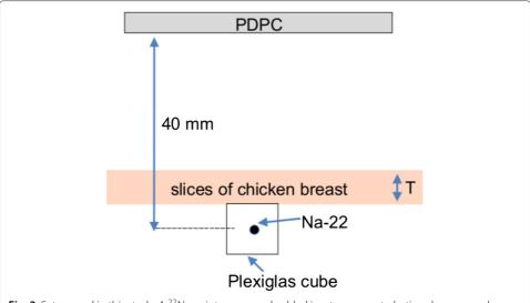
**Fig. 3** Setup used in this study. A  $^{22}$ Na point source embedded in a transparent plastic cube was used as a Cherenkov radiator, and tissue slices of different thickness (T = 2-9 mm) were used as an attenuator
