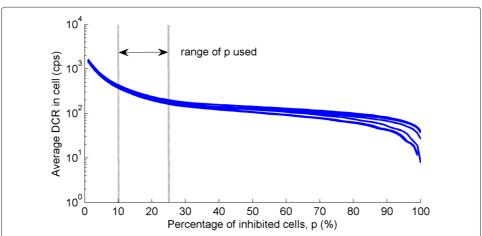
**Fig. 7** Dark count rate dependence on tile inhibited area. Average dark count rate in a cell of the PDPC as function of the percentage of inhibition p, for all the DCMs acquired at different temperature in the range (10-13) °C (different curves)
