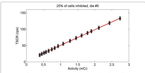
**Fig. 15** Linearity of count rate with activity. TSCR measured in one central die as a function of the source activity at the time of the measurements (*circle*). Linear fit of Eq. 4 (*solid line*)
