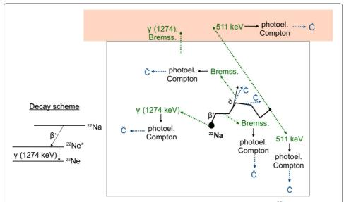
**Fig. 1** Physics processes resulting in Cherenkov radiation emission. *Left* decay scheme of  $^{22}$ Na. *Right* different processes that result in Cherenkov radiation emission: in the source container (*bottom*) and in the external layer of arbitrary thickness (*top*). Abbreviations, *Bremss* Bremsstrahlung, *photoel* photoelectric effect,  $\delta = \delta$  ray,  $\check{C} = \text{Cherenkov radiation}$
