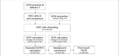
**Fig. 6** Data processing flow. Procedure for dark count maps (*left*), and for source count maps (*right*). Acronyms, *DCM* dark count map, *SCM* source count map, *p* percentage of inhibition (fraction of HDC cells discarded), *DCR* dark count rate, *SCR* source count rate, *T* average die temperature
