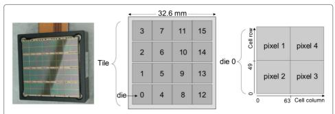
**Fig. 2** Picture and scheme of the PDPC tile. Scheme adapted from [28]. *Center* The tile is composed of 16 dies arranged in a  $4 \times 4$  matrix. *Right* Each die is composed of 4 pixels in a  $2 \times 2$  matrix. Each pixel is made of  $64 \times 50$  cells, for a total of 204,800 cells in the entire tile
