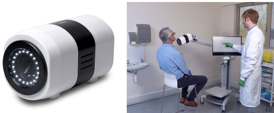
Fig. 1 Left: Seracam camera Right: Seracam system. The camera is mounted on a trolley with an articulated arm, data acquisition and display is through the integrated PC with touchscreen display
