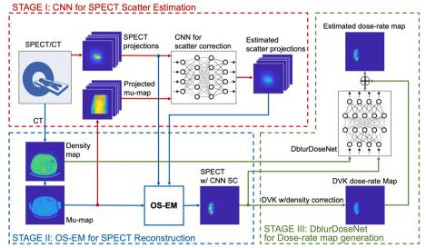
**Fig. 1** Overview of deep learning framework for 90Y Bremsstrahlung SPECT scatter estimation and voxel dosimetry. Our framework consists of (1) a deep learning model for 90Y-SPECT/CT scatter estimation; (2) SPECT reconstruction with the deep learning-based scatter estimate; (3) a residual learning network for 90Y dose estimation, trained using high-resolution virtual phantoms
