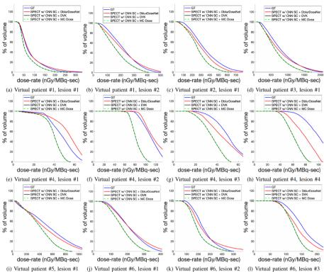
**Fig. 7** Lesion-specific cumulative dose-rate volume histograms (DRVH) corresponding to the proposed framework and MC/DVK dosimetry methods starting with the SPECT reconstruction with CNN SC
