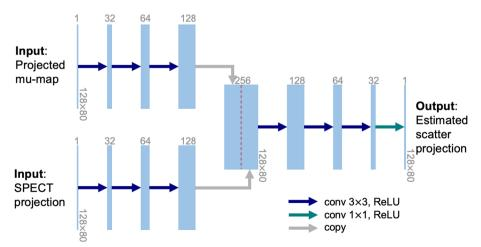
**Fig. 2** Architecture of CNN for 90Y Bremsstrahlung scatter estimation in SPECT projection space. Each blue box corresponds to a multi-channel (the number of channels is listed on the top of each box) feature map. The spatial dimensions are maintained at 128 × 80 through the entire network
