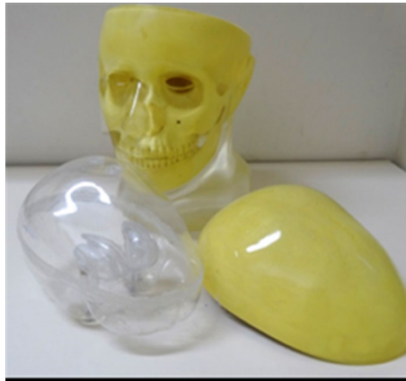
Fig. 1 Striatal anthropomorphic phantom Alderson RSD and skull to attenuation correction in equivalent tissue
