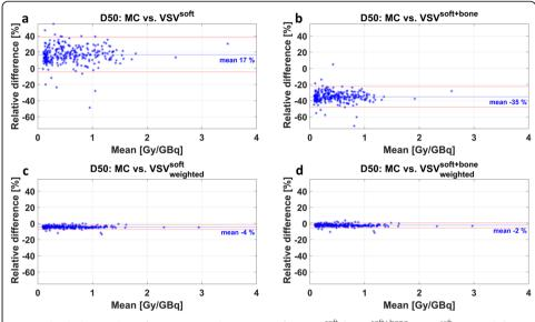
**Fig. 4** Bland-Altman plots of D50 compared against MC for **a** VSV<sup>soft</sup>, **b** VSV<sup>soft+bone</sup>, **c** VSV<sup>soft</sup>, and **d** VSV<sup>soft+bone</sup>. The mean value of both methods was plotted against the relative difference of both methods. The blue line gives the mean relative differences and the red lines indicate the 95% limits of agreement
