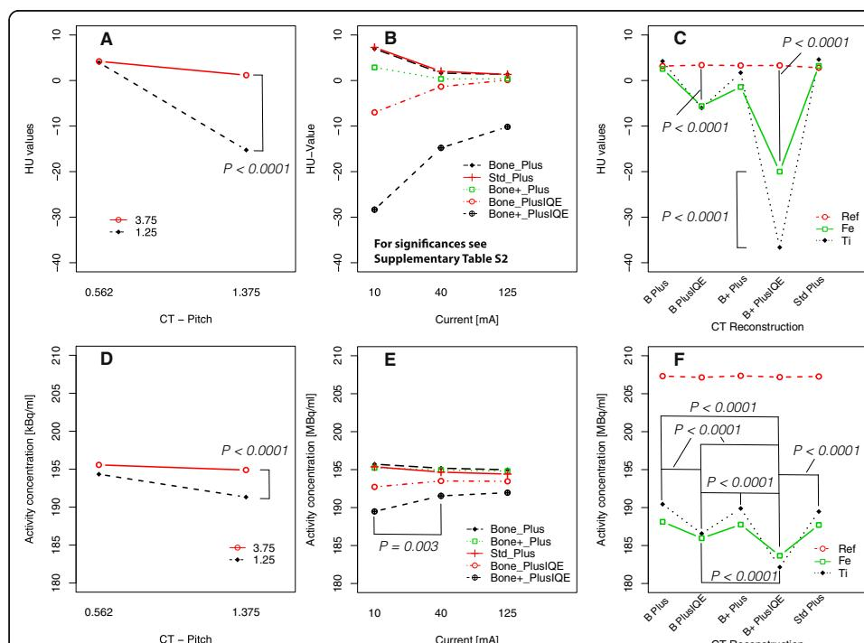
**Fig. 5** Interaction plots illustrating the effect from **a, d** pitch and reconstructed slice thickness, **b, e** X-ray tube current and CT-reconstruction/filter setup, **c, f** analyzed region and CT-reconstruction/filter setup. Effects are shown for **a-c** HU values and **d-f** corresponding reconstructed activity concentrations
