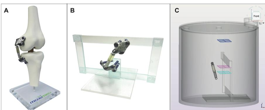
**Fig. 3** Atlas® Knee System **a** mounted to a model knee joint, **b** mounted to the acrylic frame used for positioning inside the cylindric phantom, and **c** technical drawing of acrylic frame with load absorber inserted in the phantom (analyzed ROI positions are visualized, turquoise: lateral tibia head, magenta: femur head, dark blue: reference region). The view on the phantom (CAD-drawing) is from an anterior lateral position (plates and screws of the load absorber were not visualized)
